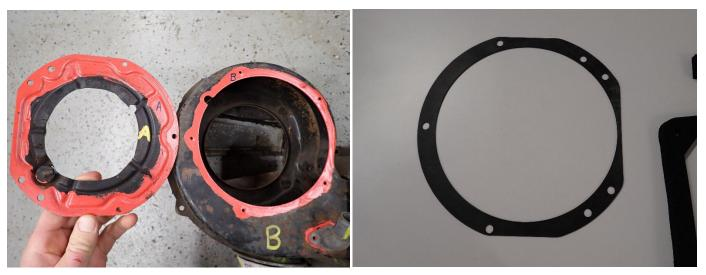
Part "A" is the actual blower motor (the picture only shows the flange of the blower motor). The seal on the right goes between the blower motor and the blower motor housing.
