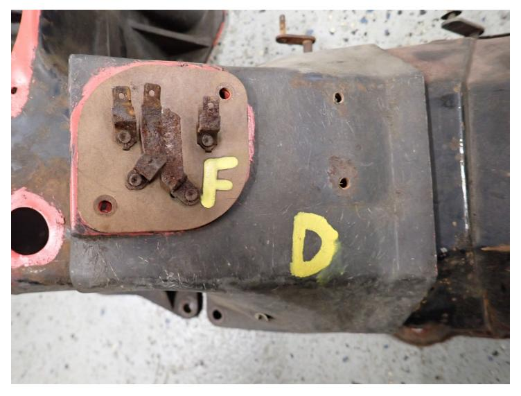
Part "D" is a fiberglass housing. Part "D" is what you need to cut and install the buytl onto. The butyl goes between the fiberglass housing and the metal blower motor housing in the left of the picture above and between the fiberglass housing and the metal heater core cover in the right of the picture above.
